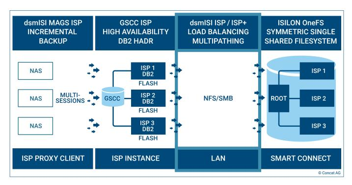
In principle, dsmISI ISP implements dynamic multipathing, which automatically spreads reads and writes symmetrically across all available network paths and Isilon nodes, guaranteeing maximum throughput for any attached ISP server. dsmISI is installed on the operating system – such as Linux, Unix or Windows – as a daemon/service and communicates with OneFS clusters, creates NFS/SMB connections to all nodes and presents them to ISP servers as a single, very fast file system.
