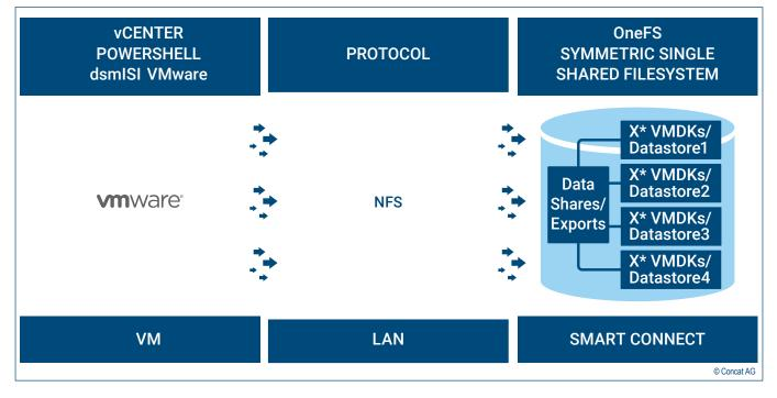
dsmISI for VMware enables organizations to integrate VMware and PowerScale (OneFS scale-out NAS) in an almost fully automated manner.
